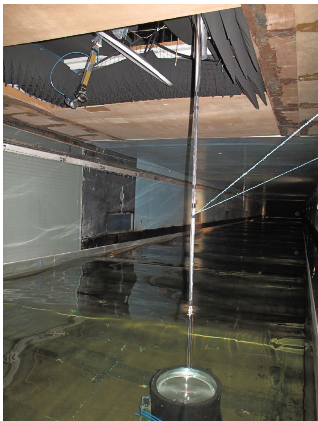
Figure 2. View of the wind tunnel, the parabolic antenna, the open waveguide, and the radar source fixed at the end of a sidearm adjusted in a crosswind azimuthal position. The whole radar system is mounted on two rotating plates set up above the tunnel roof opening and surrounded by radar absorbers. The wave gauges and the optical receiver of the slope measuring device immersed in water can be seen on the right side of the radar section.
